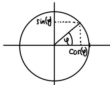
$$\text{rot}_{\varphi}(x) = \cos(\varphi)x + \sin(\varphi)y$$
